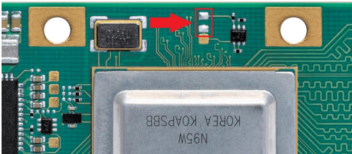
Figure 20 Location of recovery mode pads
