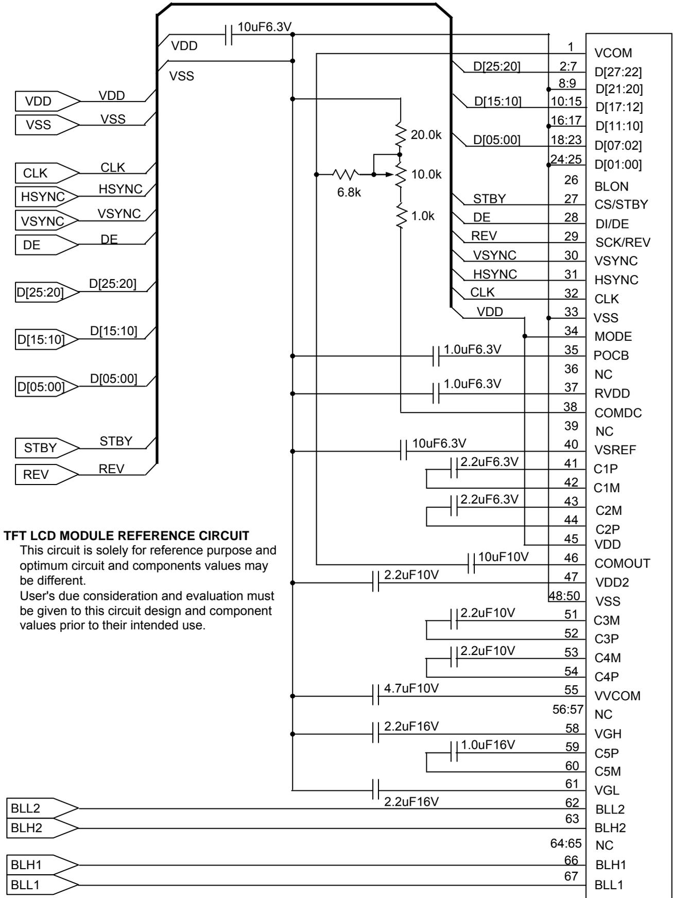
**TFT LCD MODULE REFERENCE CIRCUIT**
