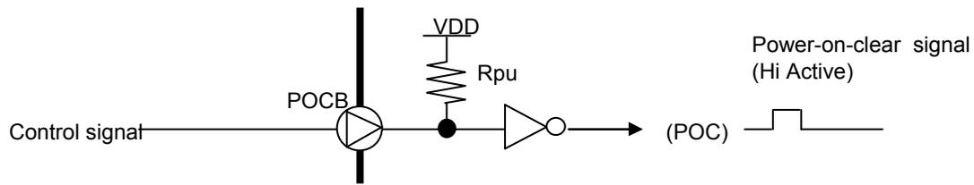
In case of directly controlling POCB terminal, POCB terminal should be set to "Lo" at Power-on. POCB should be changed to "Hi" after VDD is exceeding 2.7V. Serial communication is prohibited while POCB is "Lo".
