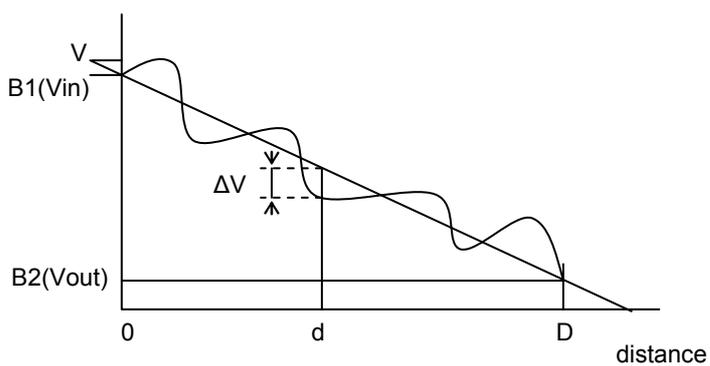
$$LE(\%) = \frac{\Delta V}{(V_{in} - V_{out})} \times 100$$
