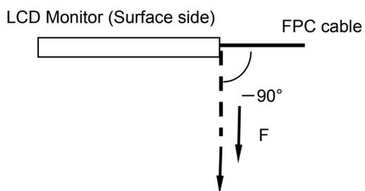
Bend Test Method for FPC cable
