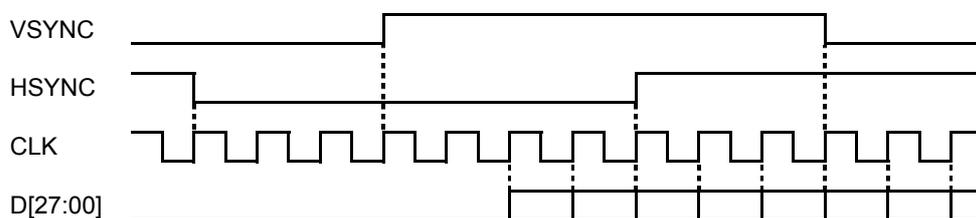
Example 3 : DI4=DI5=1, DI6=0 (CLK is reversed, data is read at the rising edge of CLK.)
