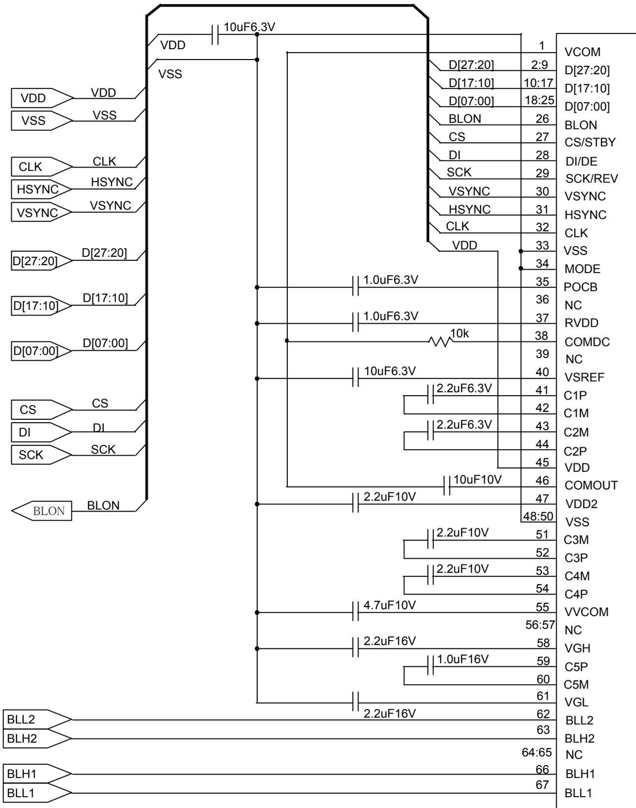
**TFT LCD MODULE REFERENCE CIRCUIT**
