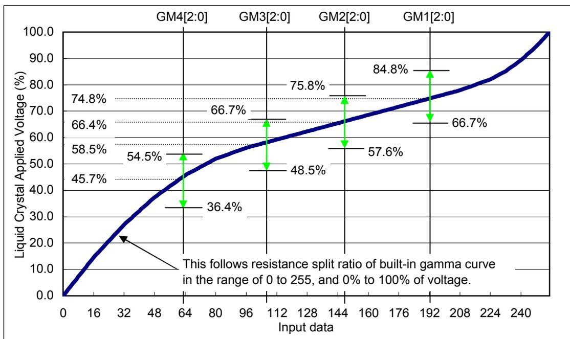
When no correction is made to gamma potential of GM1 to GM4;
