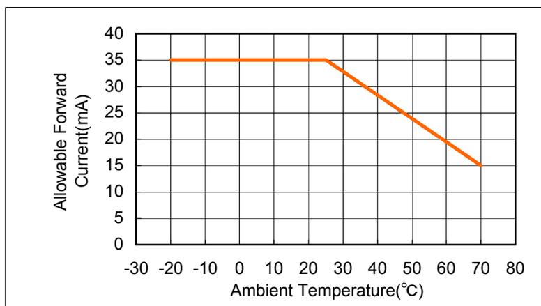
Fig. 2: Allowable Forward Current
