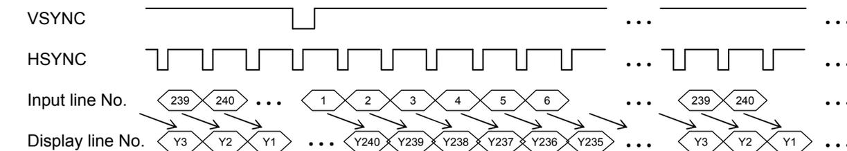
\* Above timing chart shows correlation between input data and pixels in visual way and it is not actual timing chart.
