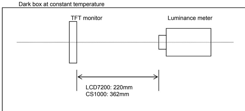
Measurement is made after 30 minutes of lighting of the backlight.
