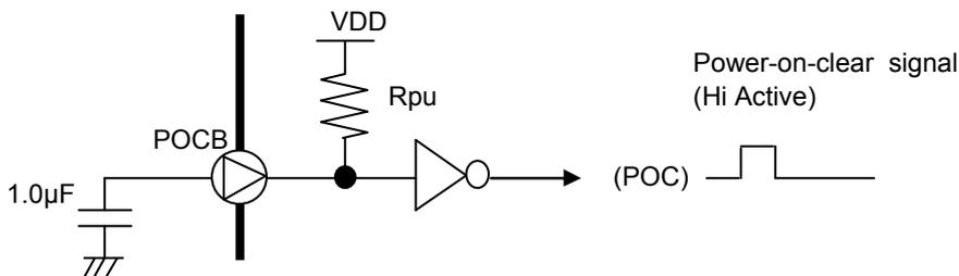
POCB terminal is connected to VDD through the pull-up resistor (Rpu).
