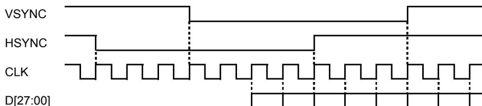
Polarity of each signal can be changed independently by logic of DI4, DI5 and DI6.
