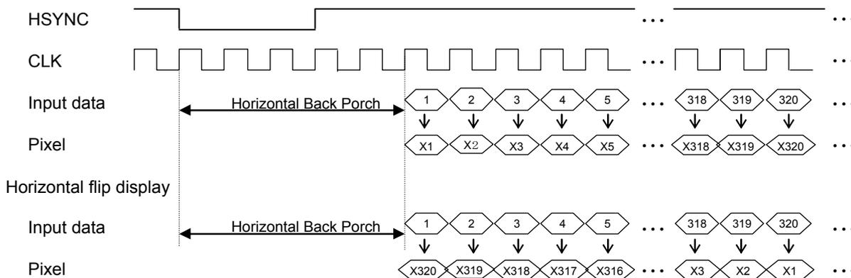
\* Above timing chart shows correlation between input data and pixels in visual way and it is not actual timing chart.
