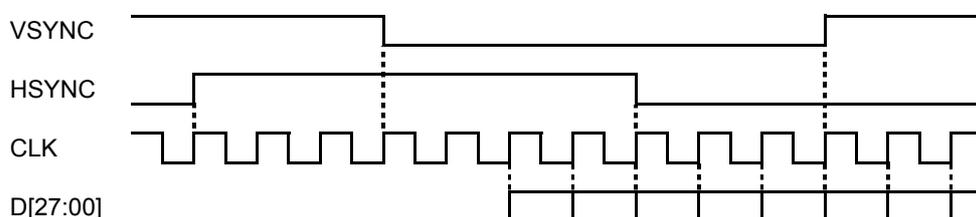
Example 2 : DI4=1, DI5=0, DI6=1 (VSYNC has positive polarity and Hi active)
