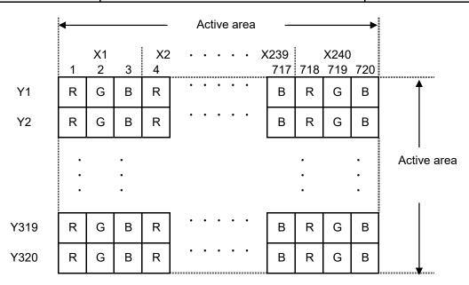
Fig. 1: Dot arrangement (FPC cable placed left)
