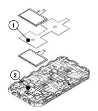
Step1: Each product is to be placed on the try with it's the displaysurface facing upward. (2 products per the first step)
