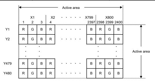
Dot arrangement (FPC cable placed down side)
