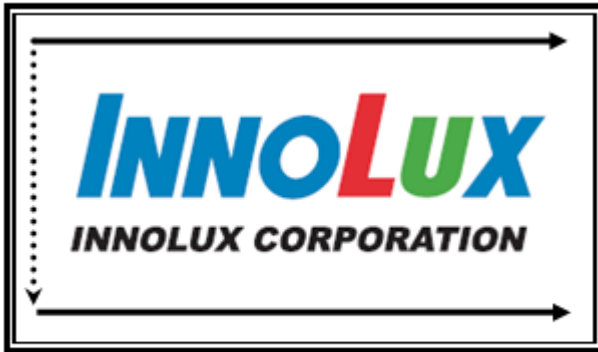
RPFI = Low/floating; normal display (default)
