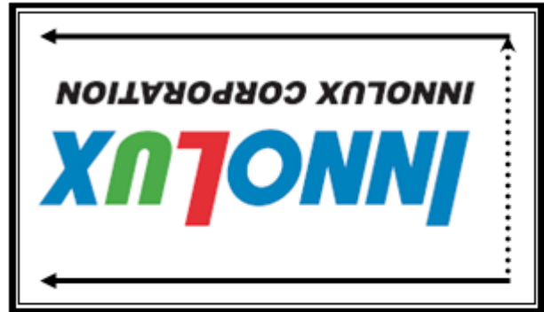
RPFI = high: display with 180degree rotation
