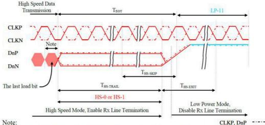
If the last load bit is HS-1, the transmitter changes from HS-1 to HS-0. If the last load bit is HS-0, the transmitter changes from HS-0 to HS-1.
