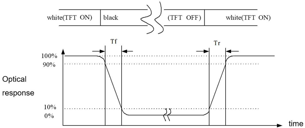
**Note (4)** Definition of optical measurement setup
