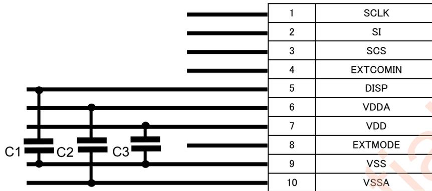
Figure 10-1 External capacitor recommendation capacity value
