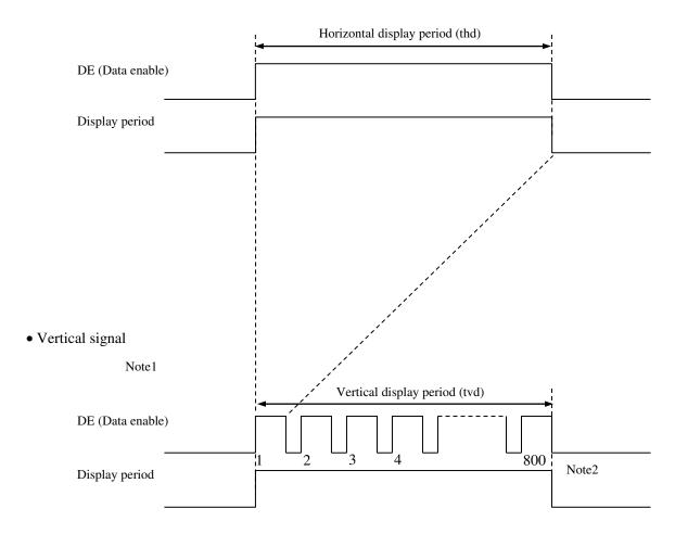
Note1: This diagram indicates virtual signal for set up to timing. Note2: See "**4.8.3 Input signal timing chart**" for the pulse number.
