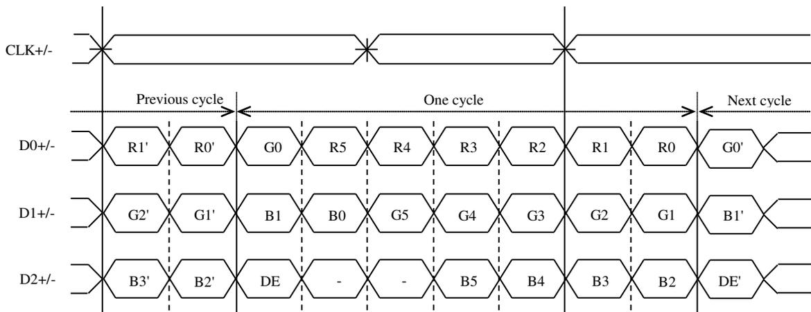
Note1: LSB (Least Significant Bit) – R0, G0, B0 MSB (Most Significant Bit) – R5, G5, B5
