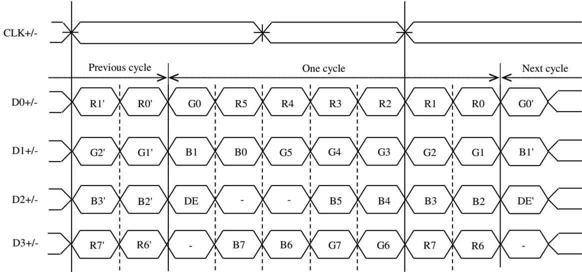
Note1: LSB (Least Significant Bit) – R0, G0, B0 MSB (Most Significant Bit) – R7, G7, B7
