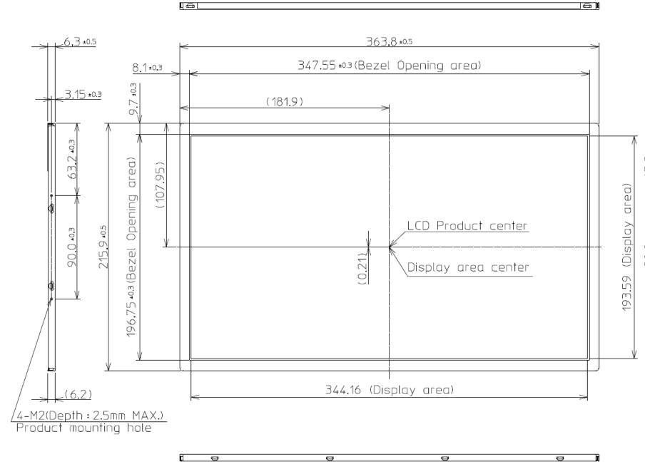
Note1: The values in parentheses are for reference. Note2: The torque for product mounting screws must never exceed 0.230 N·m. And the length of product mounting screws must be  $\leq 2.5$  mm.
