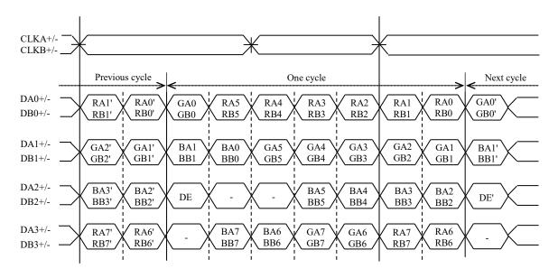
Note1: LSB (Least Significant Bit) – RA0, GA0, BA0, RB0, GB0, BB0 MSB (Most Significant Bit) – RA7, GA7, BA7, RB7, GB7, BB7
