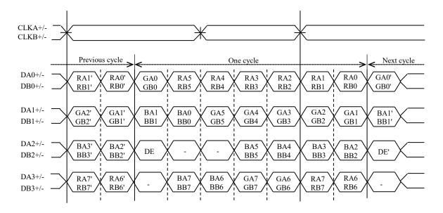
Note1: LSB (Least Significant Bit) – RA0, GA0, BA0, RB0, GB0, BB0 MSB (Most Significant Bit) – RA7, GA7, BA7, RB7, GB7, BB7
