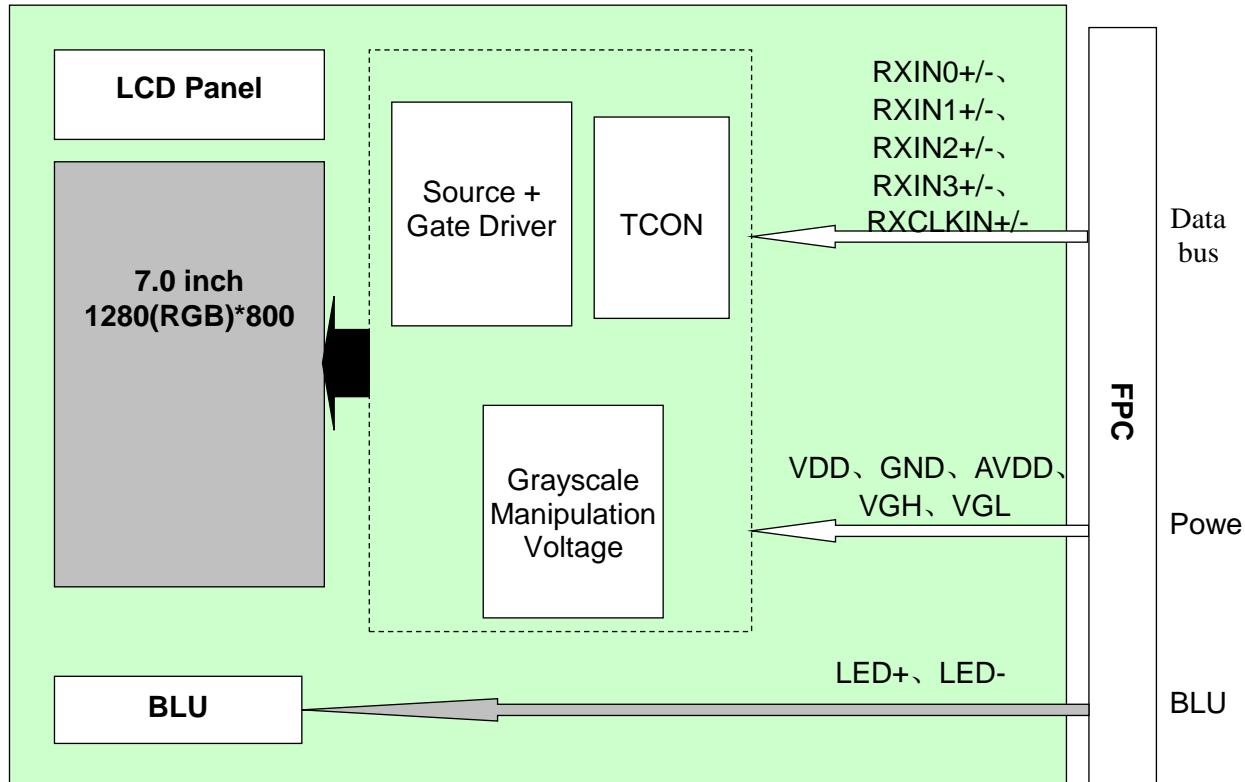
Figure 5.4.1 TFT Block Diagram
