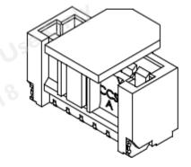
DIM.  $A = 1.00 \times NO$ . OF SPACES DIM. B = DIM. A + 2.90DIM. C = DIM. A + 1.50\* AVAILABLE IN 2 THROUGH 20
