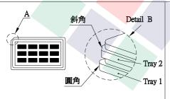
4.TRAY盤相疊時,需旋轉180度,請詳見B視圖 Rotate tray 180 degrees and place on top of stack. Check the tray stack using Fig. B.
