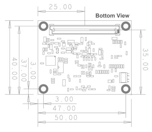
Figure 2: Mechanical Dimensions [mm]
