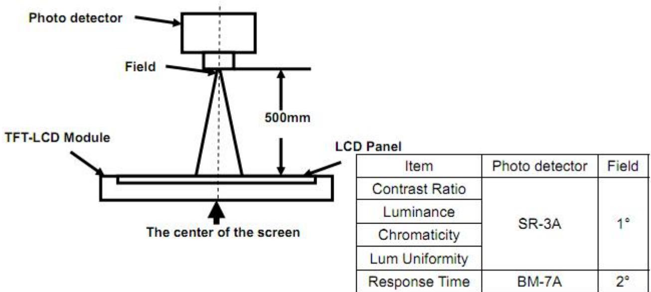
Note 2: Definition of viewing angle range and measurement system.
