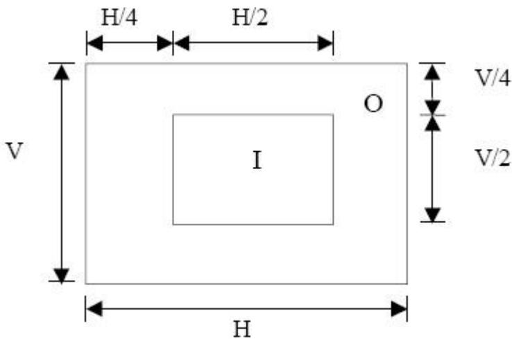
Note: 1). Dot defect is defined as the defective area of the dot area is larger than 50% of the dot area.
