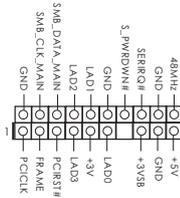
This connector supports Trusted Platform Module (TPM) system, which can securely store keys, digital certificates, passwords, and data. A TPM system also helps enhance network security, protects digital identities, and ensures platform integrity.
