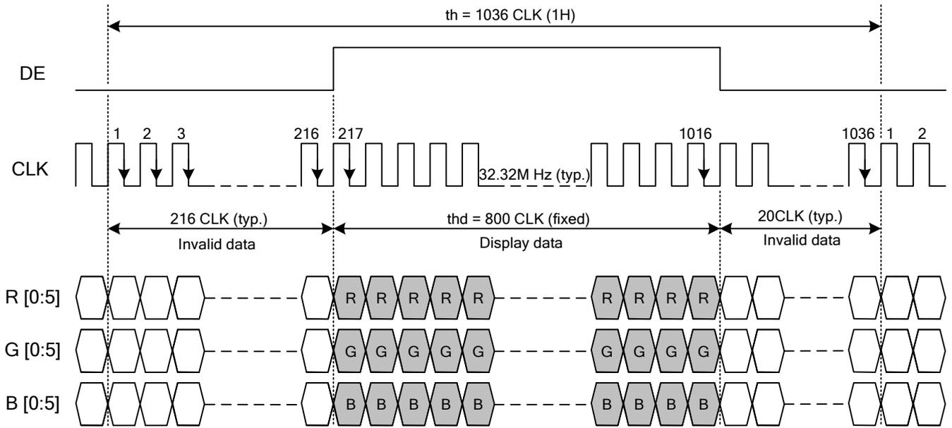
Fig. 9.3 Horizontal Timing
