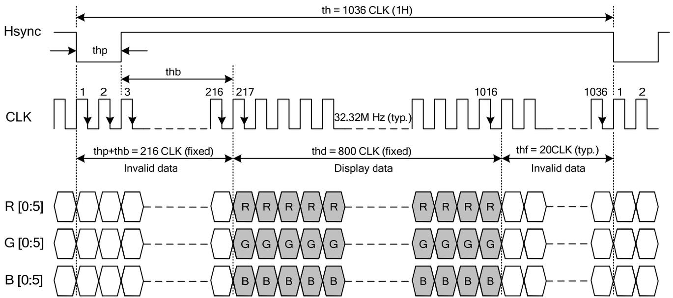
Fig. 9.1 Horizontal Timing
