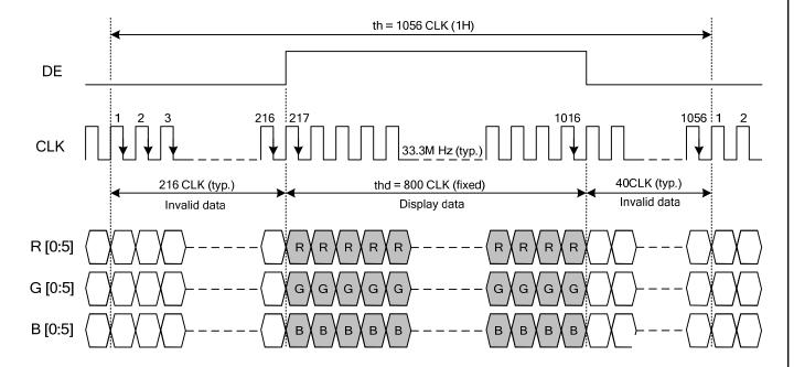
Fig. 9.1 Horizontal Timing
