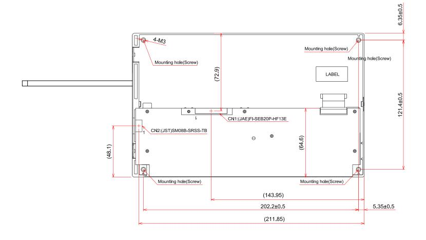
Note 1: Maximum length of screw for the mounting hole is 3.3mm
