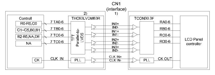
Note 1:  $100 \Omega$  impedance of LVDS cable is recommended for best optical performance.
