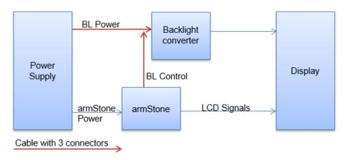
Figure 4: backlight connection with single cable
