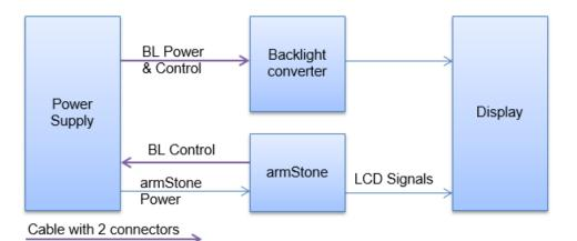
Figure 5: backlight connection with 2 cable
