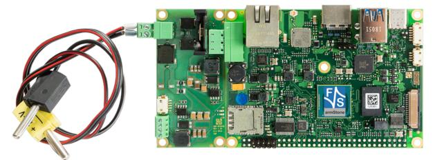
The extension board is designed to plug it into the power Connector of the armStone. For more information check the F&S website: https://www.fs-net.de/de/produkte/zubehoer/power-adapter-2/
