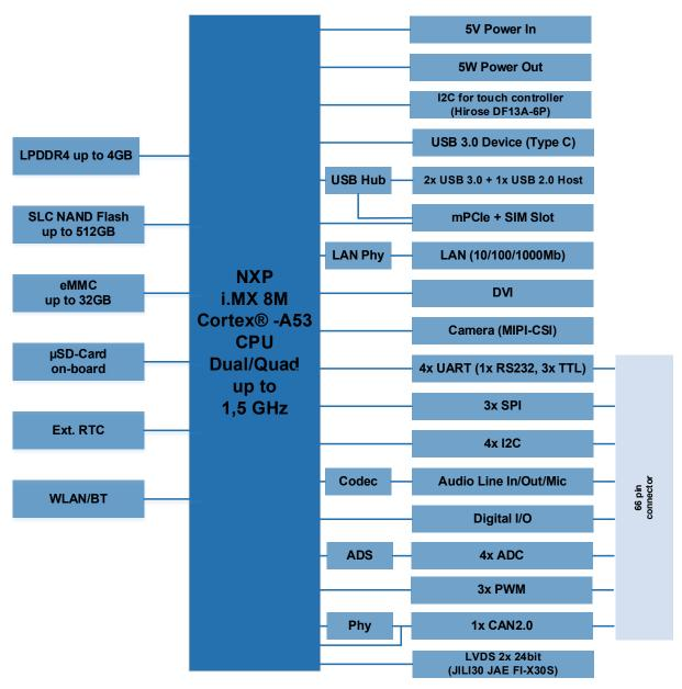
Figure 1: Block Diagram
