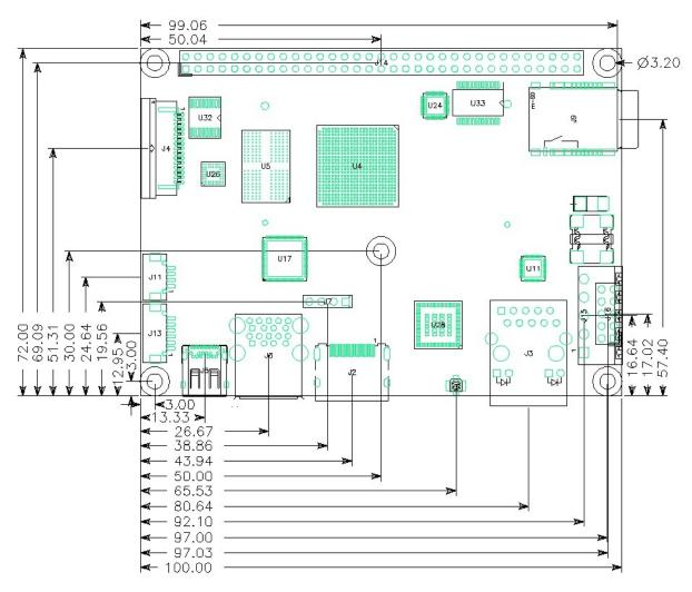
Figure 2: Mechanical Dimension Top
