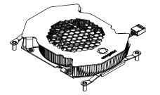
M2.5 x 10 mm threaded standoff for threaded version or ø2.7 x 10 mm non-threaded standoff for borehole version
