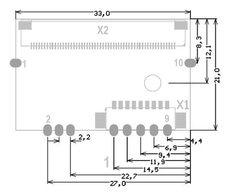
all Dimensions in mm (Tolerance +/- 0,3 mm)
