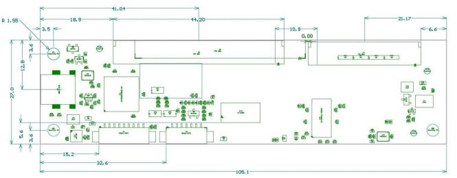
Height: 6mm (including components) All dimensions in mm
